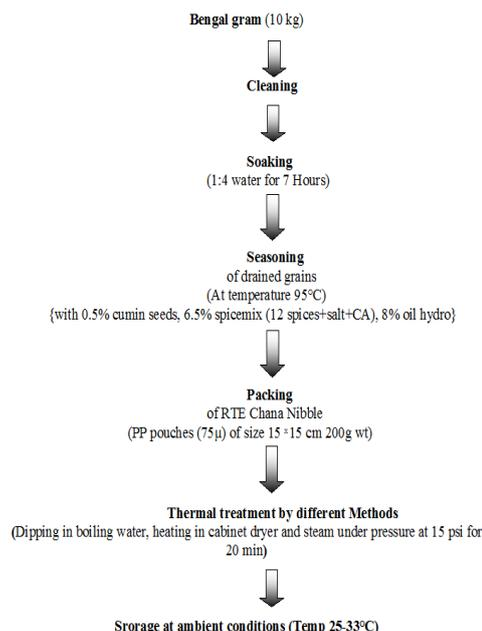
Figure 1. Process flow Chart for the preparation of RTE Chana Nibble
